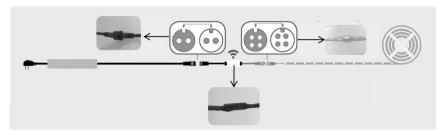
Middle: Receiver Remote control Left: black connection to power supply (2-pin plug) Right: transparent connection to the pool (4pin plug)
