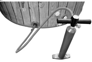
9. Once inflated turn anti-clockwise to release inflation hose and replace valve cap.
