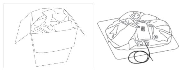
• Open the air outlet on top of the filter heating element of the whirlpool and screw on the filling hose.
