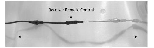
Left: black connection to power supply (2-pin plug) Right: transparent connection to the pool (4-pin plug)
